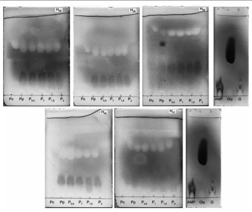
Fig. 1. The TLC chromatograms of fermentation broths of the tested fungi of *Fusarium* species after three weeks of incubation. Used standards: AMPA– aminomethylphosphonic acid, Gly–glycin and G-glyphosate. Tested strains: H<sub>38</sub>, H<sub>39</sub> – *F. solani*, H<sub>40</sub> – *F. moniliforme*, H<sub>41</sub> – *F. oxysporum*, H<sub>65</sub> – *F. sporotrichioides*
